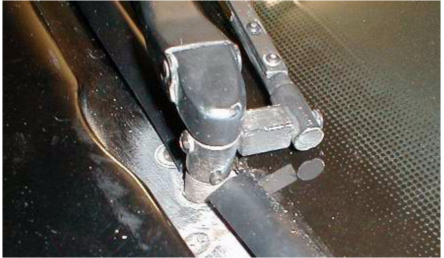
Windshield wiper installed
