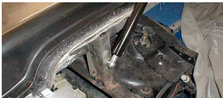
FIGURE 114. Body shock mount for motor deck lid
