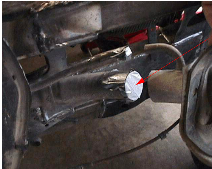
FIGURE 30. Gas tank filler and vent cut
