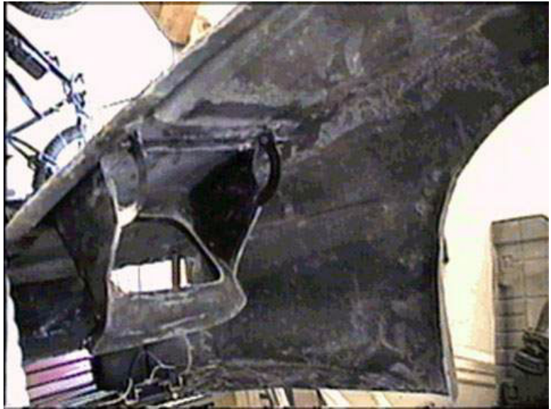
FIGURE 73. Bracket installed - view from under fender well
