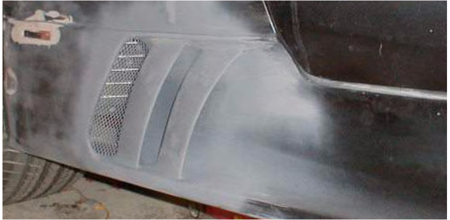
FIGURE 68. Final louver assembly
