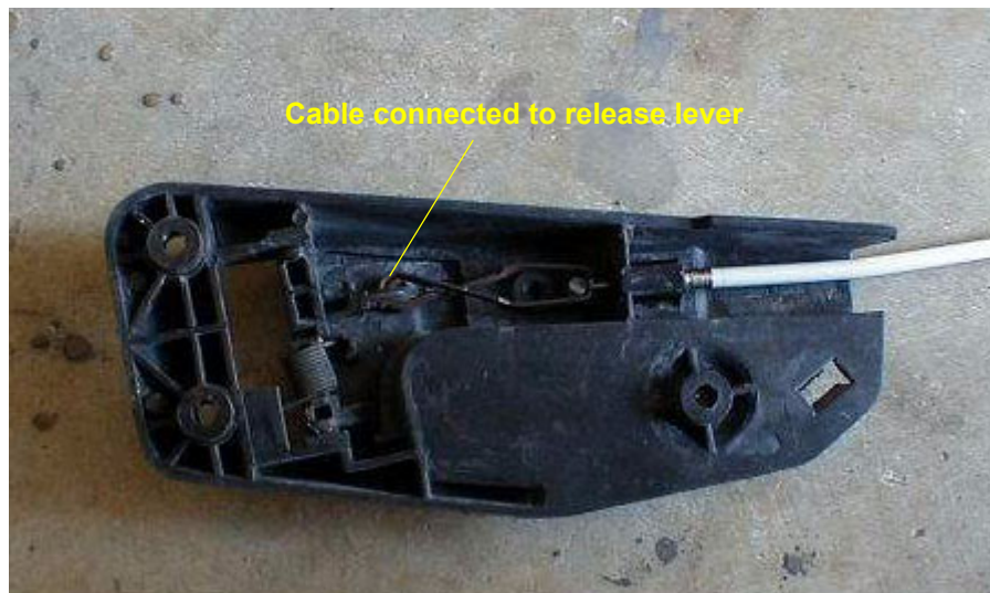
FIGURE 57. Completed interior latch assembly
