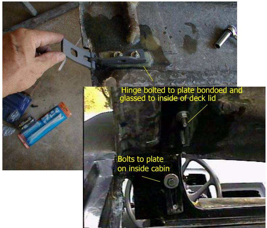
FIGURE 109. Deck lid hinge detail
