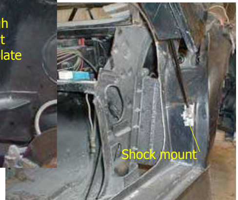
FIGURE 89. Completed body shock plate mount
