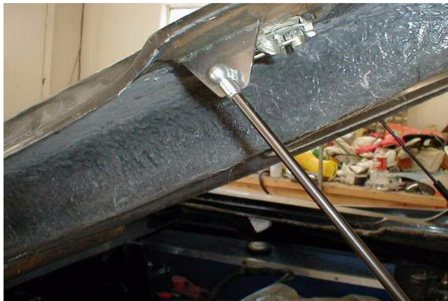
FIGURE 113. Upper shock mounted on motor deck lid
