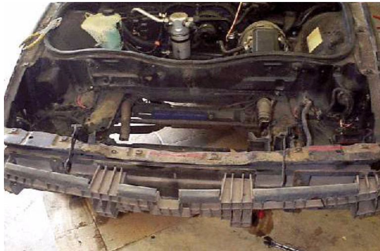
FIGURE 43. Front of car with radiator removed
