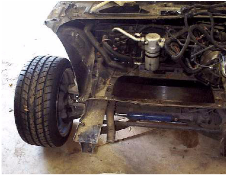
FIGURE 45. Front view after fenders have been removed
