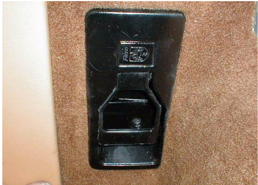
FIGURE 179. Finished roof release mechanism
