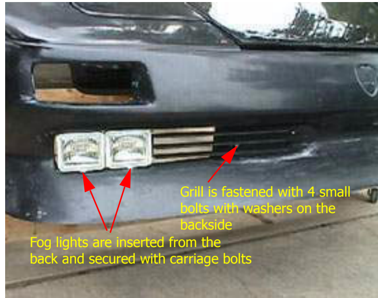
FIGURE 62. Fog Lights and Grills installed
