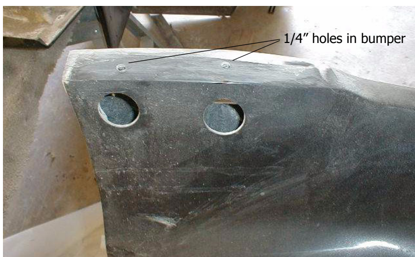
FIGURE 125. Side bumper mounting holes
