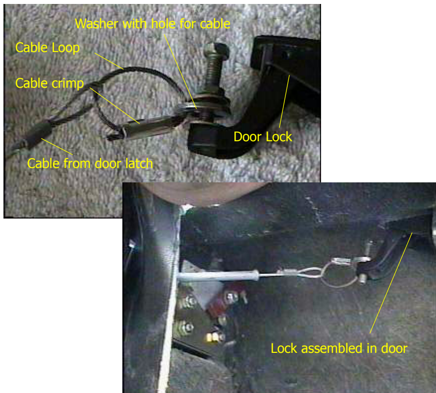
FIGURE 91. Completed door lock assembly
