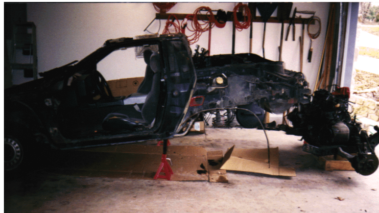
FIGURE 3. Donor Car with panels and Engine removed
