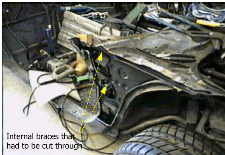
FIGURE 47. Fender after the cut
