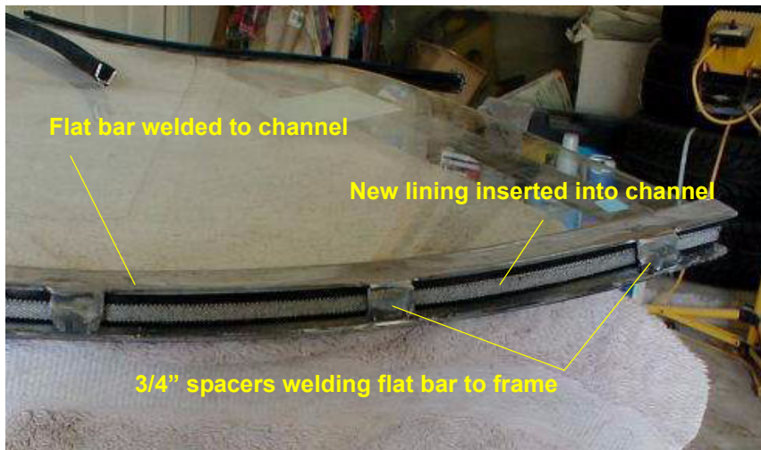
FIGURE 139. Flat bar welded to frame with new channel inserted
