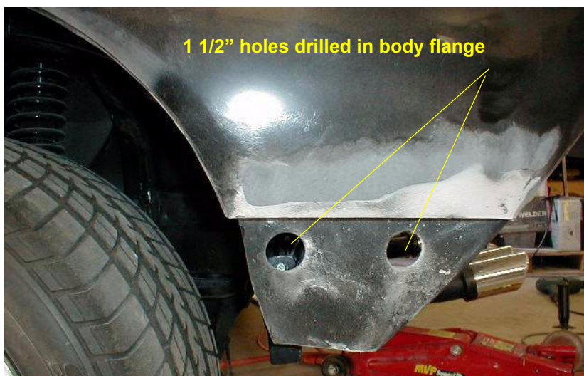
FIGURE 126. Body holes for bumper
