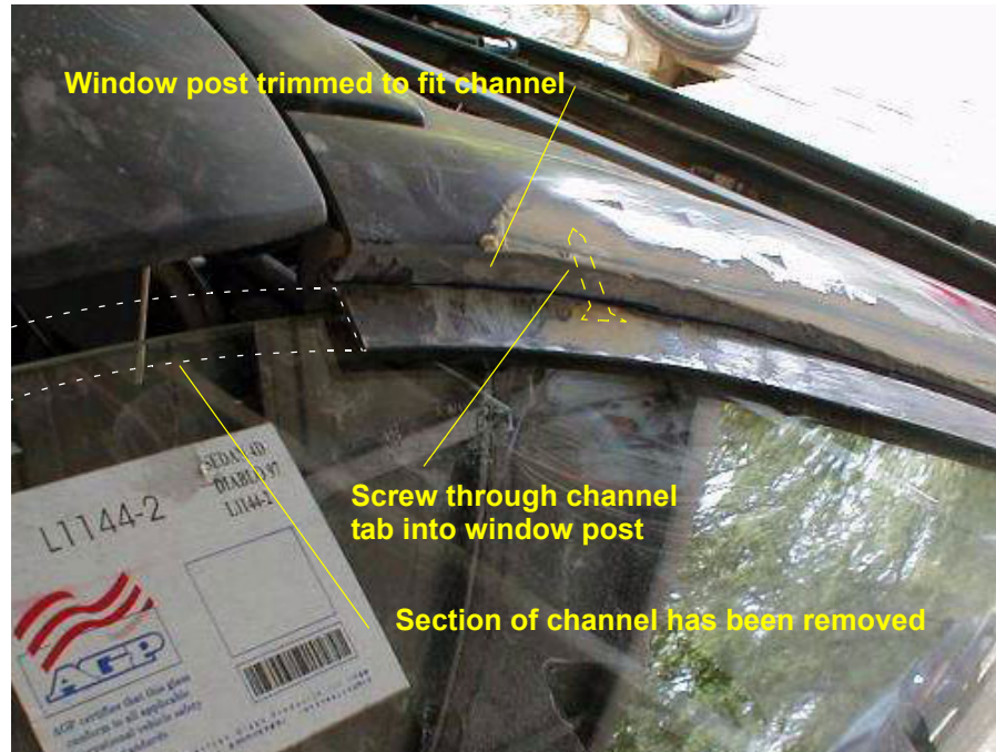
FIGURE 143. Fastening top channel to post
