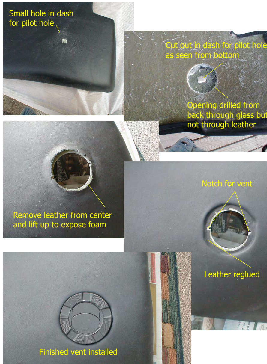
FIGURE 160. Vent installation process
