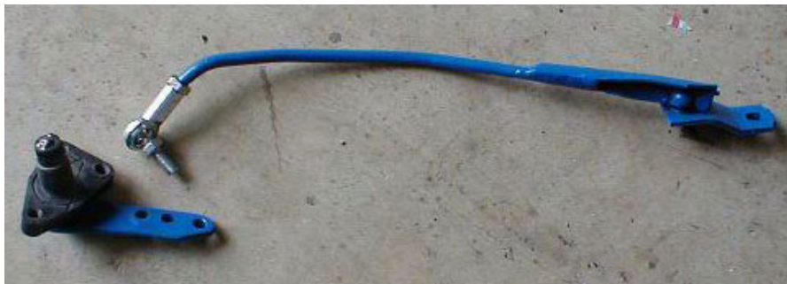
FIGURE 154. Final assembled arm components
