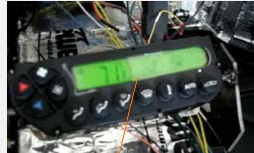
Functional OEM heater controls that operate new Vintage A/C unit
