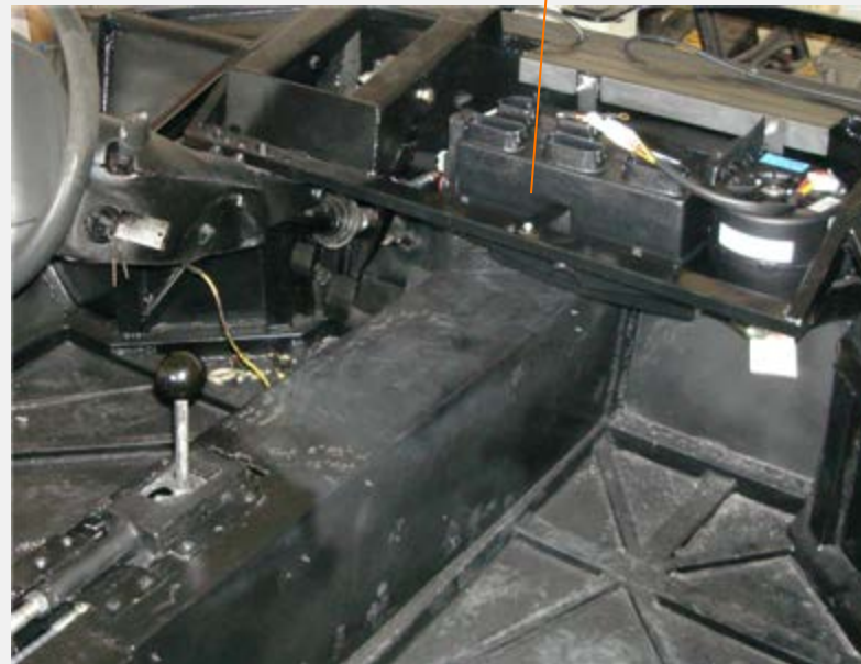
Functional OEM heater controls that operate new Vintage A/C unit
